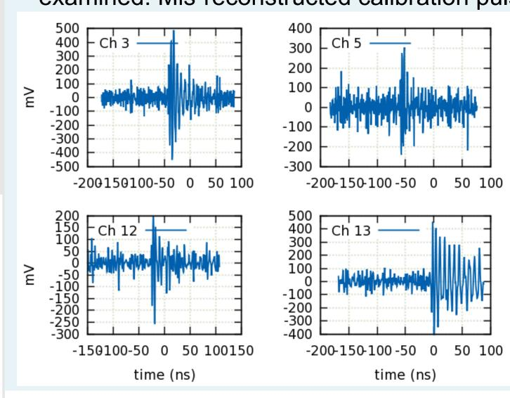
Waveforms from triggered antennas for the single passed event
